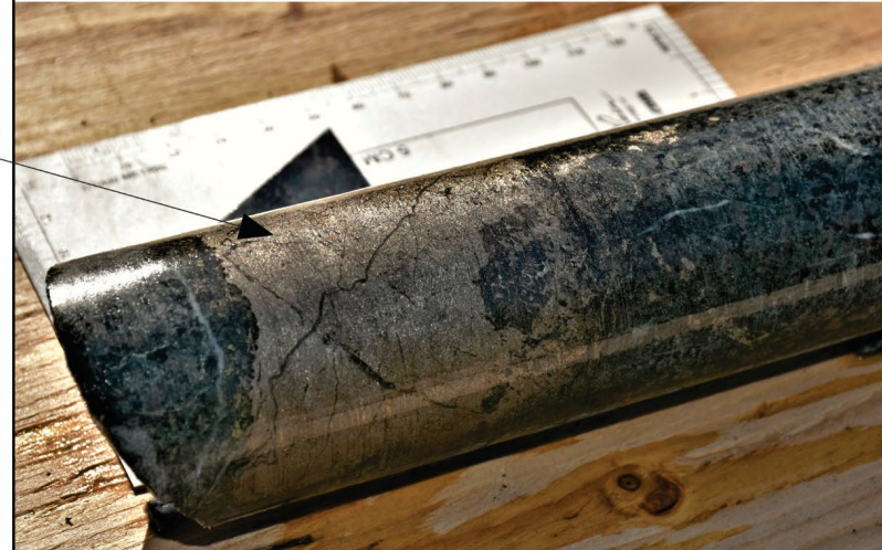
Semi massive nickel and copper bearing sulphides at 597.3m in EL-22-97b. Mineralization is hosted with well mineralized E&L gabbro with heavily disseminated to blebby, to semi massive sulphides.
